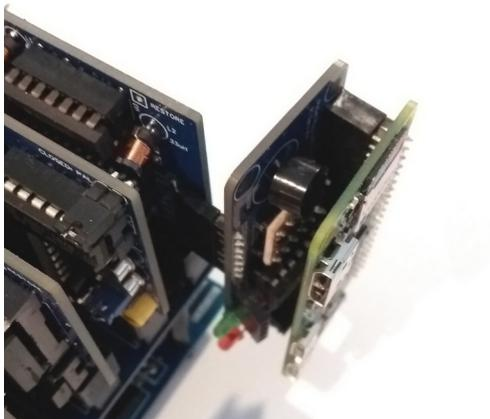
To ensure that the internal Pi1541 functions reliably, the CIA 6526 (U8) socket should be equipped with a CSG 6526/216A on the rear side if possible. According to one user, MOS 6526/216A should also work, but during my tests I already had problems with MOS 6526/216A chips. Furthermore the following files on the SD-card of the Raspberry pin should be changed.
